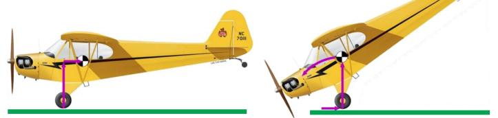
The typical way to mitigate this is to slow the plane down with the idea that the slower the plan is going, the lower the forces that will be imparted on the wheels.
