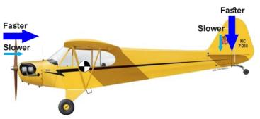
surfaces are. If you slow way down to just above stall speed, the control surfaces have only marginal effect and aren't very effective is preventing a ground loop. The slower you are going, the less effective the elevator is in keeping your tail down.
